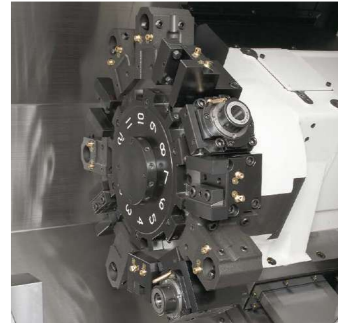
V12 radial multitasking turret (Optional)
