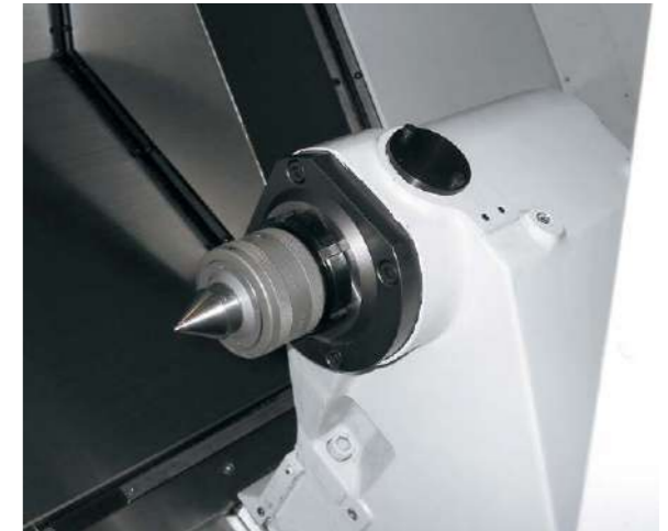
Note: Please select a hydraulic quill for face driver machining applications.
