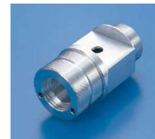
X•Y plane Radial Y-axis machining examples
