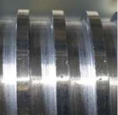
Smooth surface, clean finished threads
