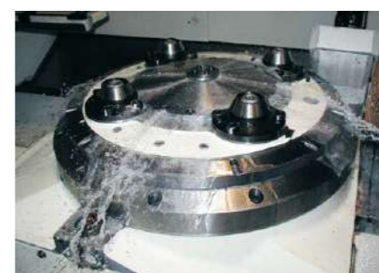
Washing with coolant under pallet
