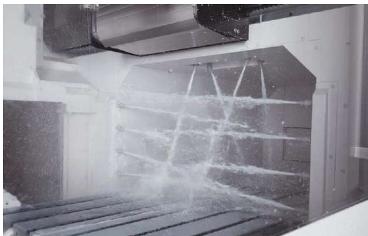
Crossrail shower system (Optional) removes chips from the workpiece and table
