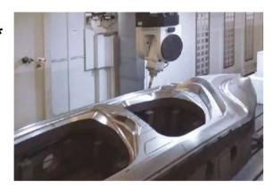
High speed continuous feed while maintaining high shape accuracy and machined surface quality
