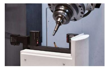
The swivel type laser sensor is mounted behind the table near the cutting point. Since the measuring device also turns with the indexing of the attachment head measurement of the cutting edge position is done while in the machining area.
