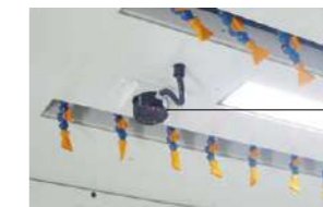
Receiver (sends and receives touch probe signals)
