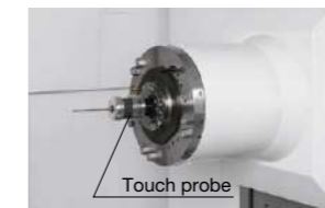
Auto zero offset and auto gauging (wireless touch probe)
