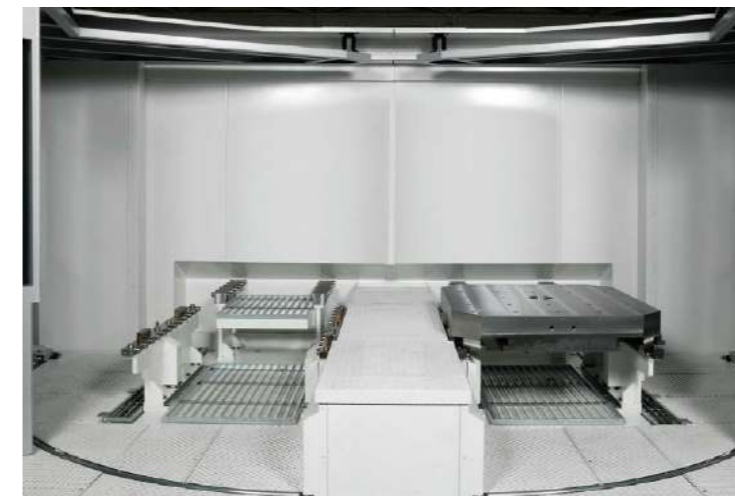
Thorough consideration of fixture workability in APC · Basically flat chamber floor for easy fixture work and cleaning · Working space provided on workpiece periphery · Crane loading is easy with large double-door opening
