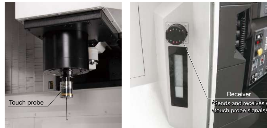
Auto zero offset, auto gauging (radio-controlled touch probe)
