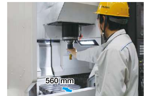
Machine front to table center 560 mm
