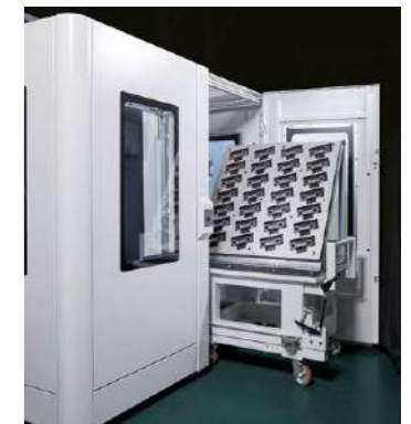
A dedicated fixture attached to the tilted cart.
